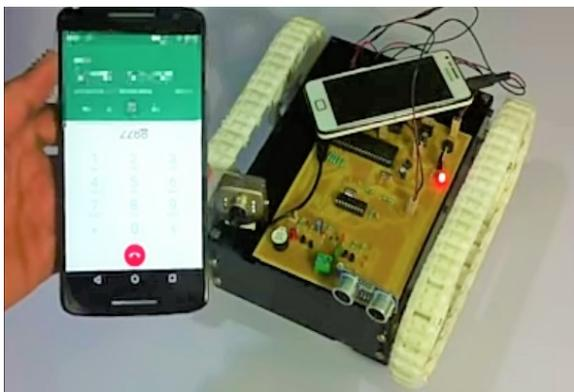
Fig -3: Cell Phone call controlled robot
